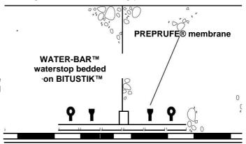
Details shown are typical illustrations only and not working drawings. For assistance with working drawings and additional technical advice please contact Allnex Construction Products.
