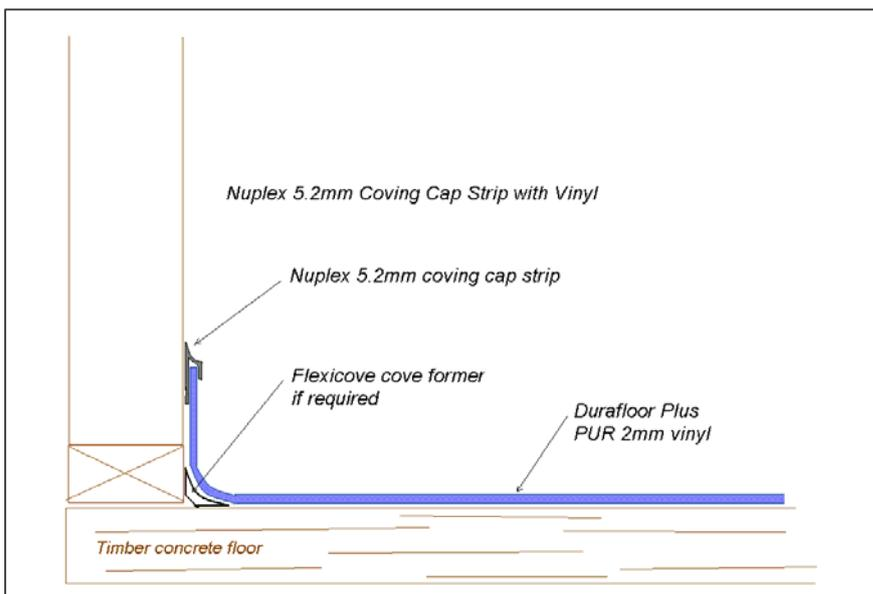
**Installation techniques and detailing of self-coved vinyl to architrave**
