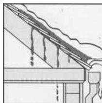
As the ice dam grows, water is trapped behind it and backs up under the shingles. Eventually it reaches the roof deck and leaks through, damaging the interior of the structure.
