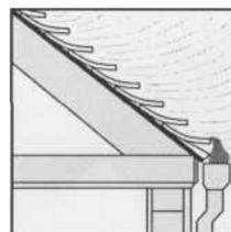
Grace Ice & Water Shield applied beneath the sloped roof covering helps prevent wind-driven rain from entering the structure.
