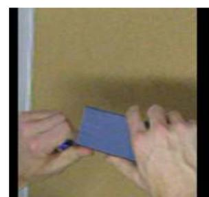
**==> Aim to loosen edge of peel-ply**
